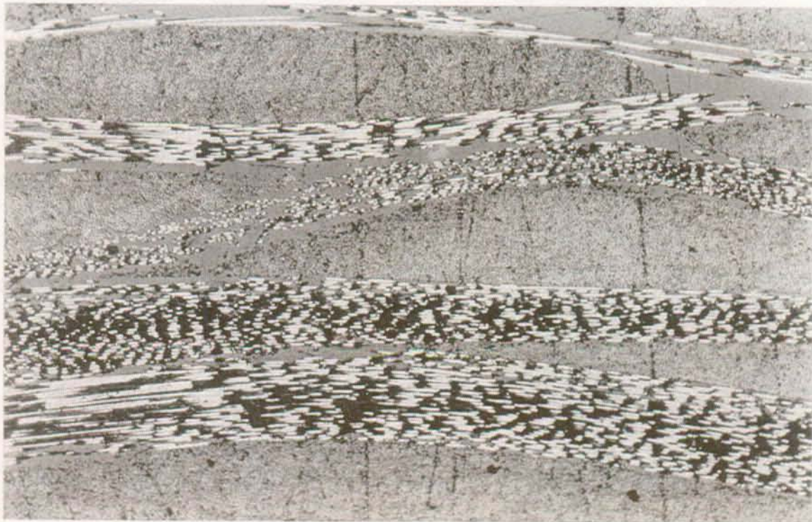
Figure 7.4: Cross section of a CF-PEEK satin 8 FIT flat laminate processed at 5 MPa (optical microscope). The waviness of the fibres and the presence of cross over points may explain the higher value of P_s when compared to UD laminates.
