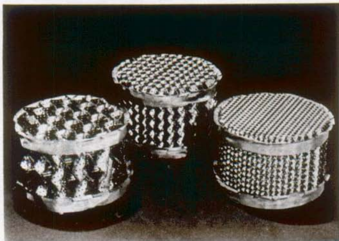
Figure 1.4 Three different types of the SULZER structured packing MELLAPAK - 125.Y, 250.Y and 500.Y.
