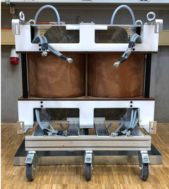
▲ 1MW prototype of the 2-vessel MFT structure
