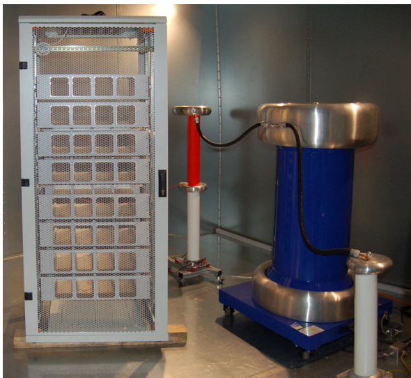
▲ Cabinet with 32 cells in Faraday cage during insulation coordination testing
