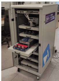
▲ Grid emulator: RT-HIL system and power HW under development (Semikron-Danfoss IGBTs, WOLFSPEED SiC MOSFETs)
