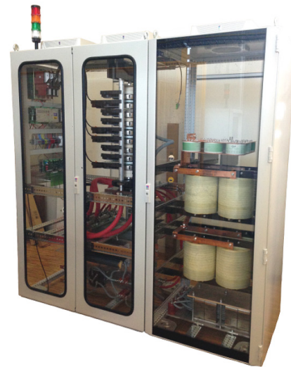
▲ Flexible and reconfigurable IGCT test setup [26]
