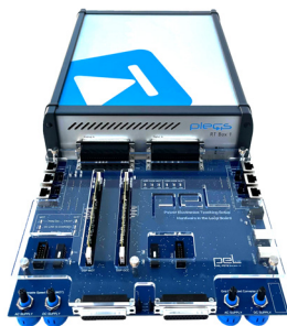
▲ Power Electronics Teaching Setup: RT-HIL system and the actual power hardware
