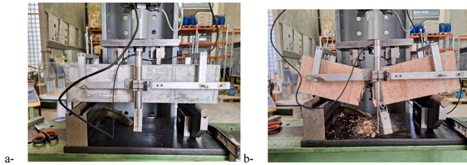
Fig. 1. Testing set-up following the AFNOR (1999) for the residual flexural strength test showing a) OPC sample before failure and b) LC<sup>3</sup> sample post-failure.
