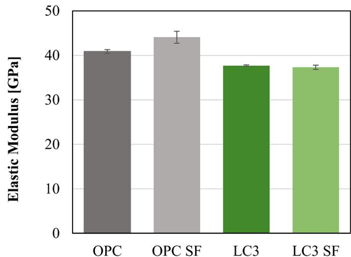
**Fig. 4.** Elastic modulus results of unreinforced and steel fibre-reinforced OPC and LC<sup>3</sup> concrete mixes.
