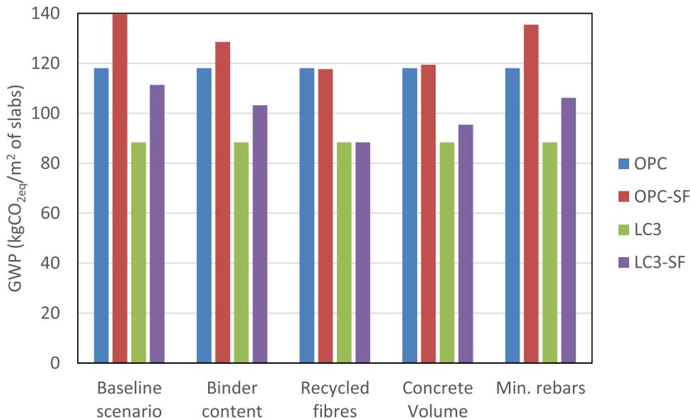
**Fig. 7.** Scenario analysis for relative decarbonization potential strategies for one-way steel fibre-reinforced LC<sup>3</sup> concrete compared to conventional steel reinforced OPC ones.
