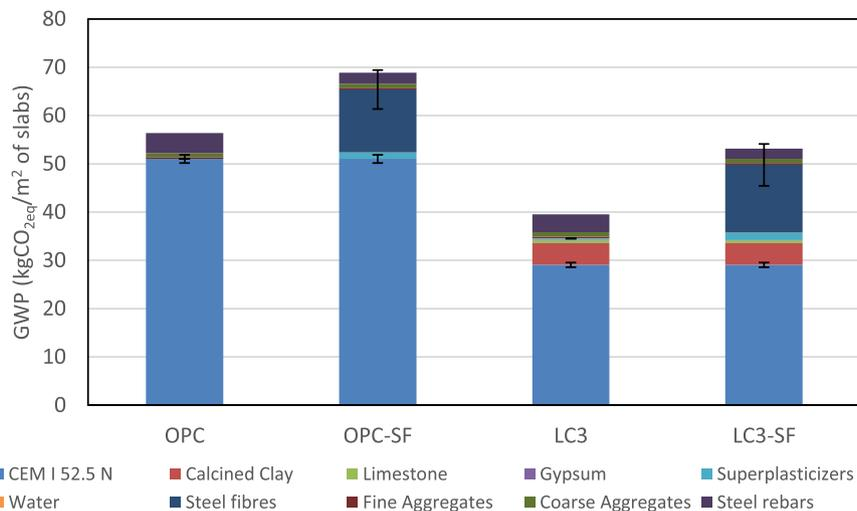
**Fig. 6.** Comparison of the carbon footprint per m<sup>2</sup> of slab of conventional vs steel fibre-reinforced OPC and LC<sup>3</sup> concrete.
