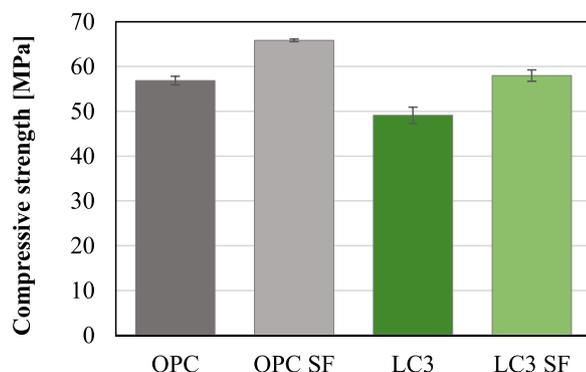
**Fig. 3.** Compressive strength results of unreinforced and steel fibre-reinforced OPC and LC<sup>3</sup> concrete mixes.
