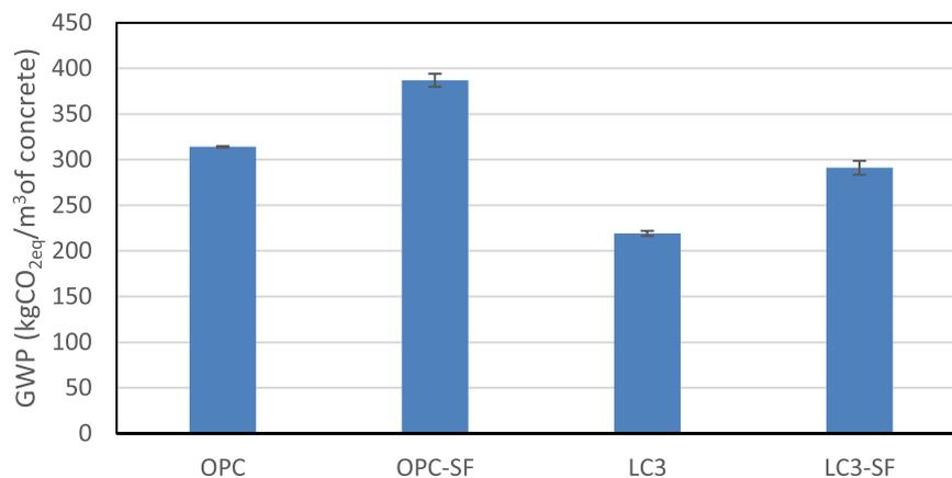
**Fig. 5.** The environmental impact assessment of OPC and LC<sup>3</sup> concrete mixes per unit volume.
