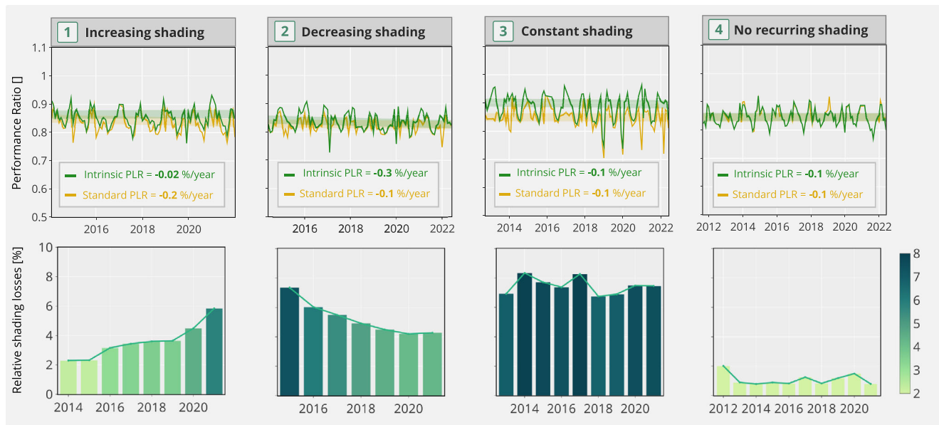
FIGURE 7 Comparison of daily performance ratio (PR) trends for the intrinsic and standard performance loss rates (PLRs) for the four identified shading loss scenarios (exemplified with different building-integrated PV [BIPV] systems), highlighting the potential shift in PR after filtering for loss factors and the impact on the PLR evaluation. Corresponding yearly relative shading loss evolution is also shown.
