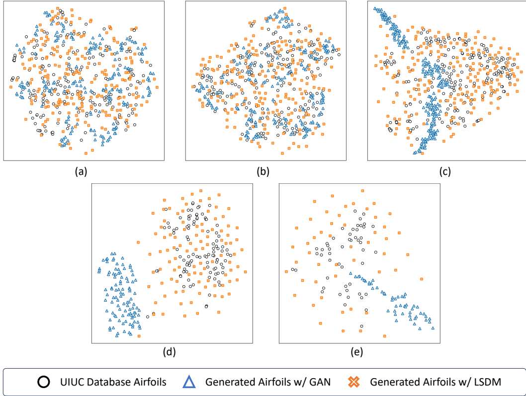
Fig. 4 The t-sne visualizations of airfoil’s latent codes from the UIUC database, LSDM and GAN, given training datasets of (a) 1000, (b) 500, (c) 250, (d) 100 and (e) 50 airfoils. Best viewed in color.
