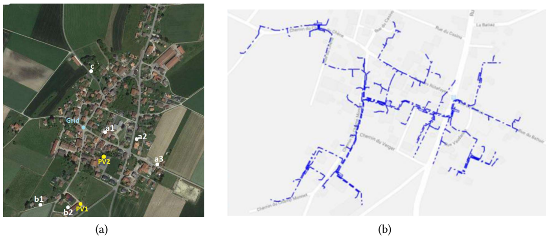
Fig. 7.15 (a) Aerial view of Chapelle-sur-Moudon (District case) with the location of the grid (blue), 6 consumers (white), and 2 PVs (yellow). (b) Actual power grid at Chapelle-sur-Moudon demo site [178].
