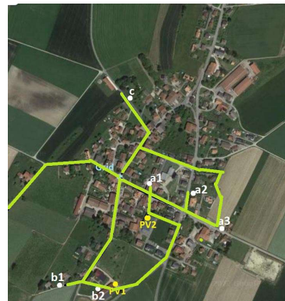
Fig. 7.17 Considered DC PDN for the district of Chapello-sur-Moudon. (a) and (b) Radial Configuration; (c) and (d) Ring Configuration; (e) and (f) Mesh Configuration. The three DC PDNs have 16 nodes, except for the ring configuration where an extra node was created between the two PV generations. Satellite photos from Google Earth.
