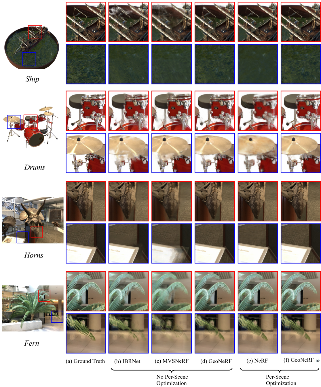
Figure 3.3: Qualitative comparison of the methods on the NeRF synthetic dataset (Martin-Brualla et al., 2021) ( Ship and Drums ) and the real forward-facing dataset (Mildenhall et al., 2019) ( Horns and Fern ). Our proposed GeoNeRF more accurately preserves the details of the scenes while it generates fewer artifacts than IBRNet (Wang et al., 2021b) and MVSNeRF (Chen et al., 2021) (e.g., the leaves in Fern or the cymbal in Drums ). After fine-tuning our model only for 10k iterations on each individual scene (GeoNeRF 10k ), the results are competitive with per-scene optimized vanilla NeRF (Mildenhall et al., 2020). Compared with NeRF, GeoNeRF models produce smoother surfaces in Drums and higher quality textures for the water in Ship and for the floor in Horns .
