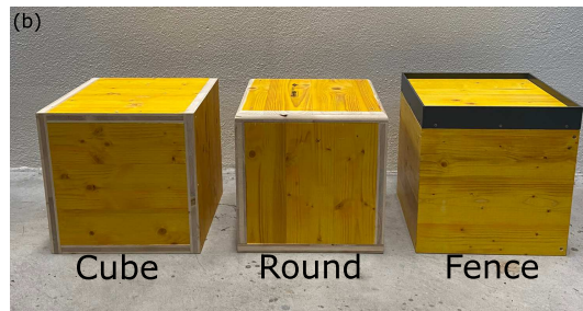
Figure 8.2: (a) Sketch of the experimental setup inside the test section; L = 8 cm, h = 10 cm and H = 40 cm. (b) A picture of the cubic tall buildings with modified roof edges.
