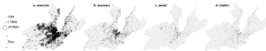
Fig. 10. Spatial distribution of material usage in terms of mass. One dot per building.
