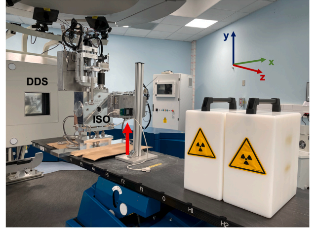
Fig. 7. Treatment room at CNAO. The red arrow indicates the device, which is placed on the patient's bed \sim 55 cm from the isocenter. The white boxes at the end of the bed are full of water and are meant to stop the beam. The two reference detectors (DDS and ISO) are also marked.
