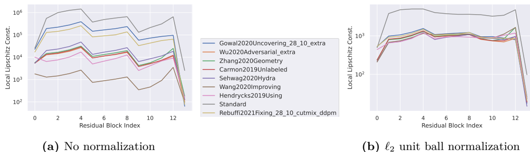
Figure 4.16: Lipschitzness. Computation of the local Lipschitz constant of the WRN-28-10 \ell_\infty -robust models in our Model Zoo with \varepsilon = 8/255 . The color coding of the models is the same across both figures. For the correspondence between model IDs (shown in the legend) and papers that introduced them, see Appendix 4.13.
