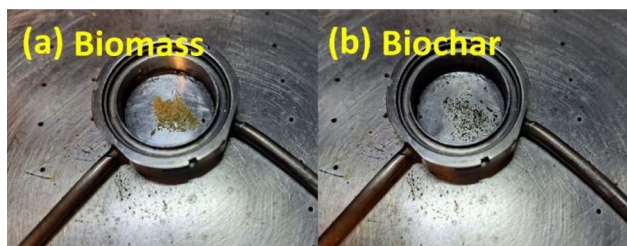
Fig. 2 (a) Overview of the biomass (feathertop plant) in the steel reactor and (b) biochar obtained after photo-pyrolysis at 575 V-pulse and flashing time of 72.5 ms.
