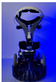
(a) Semi-autonomous wheelchair (mobile robot)
