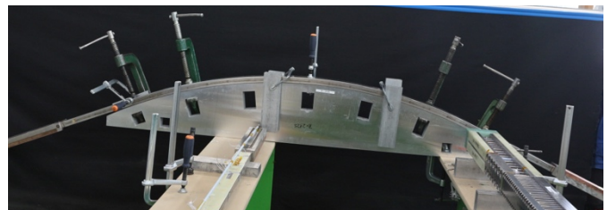
Fig. 3. Bending of the conductor section over the machined Al former at R = 1417 mm.
