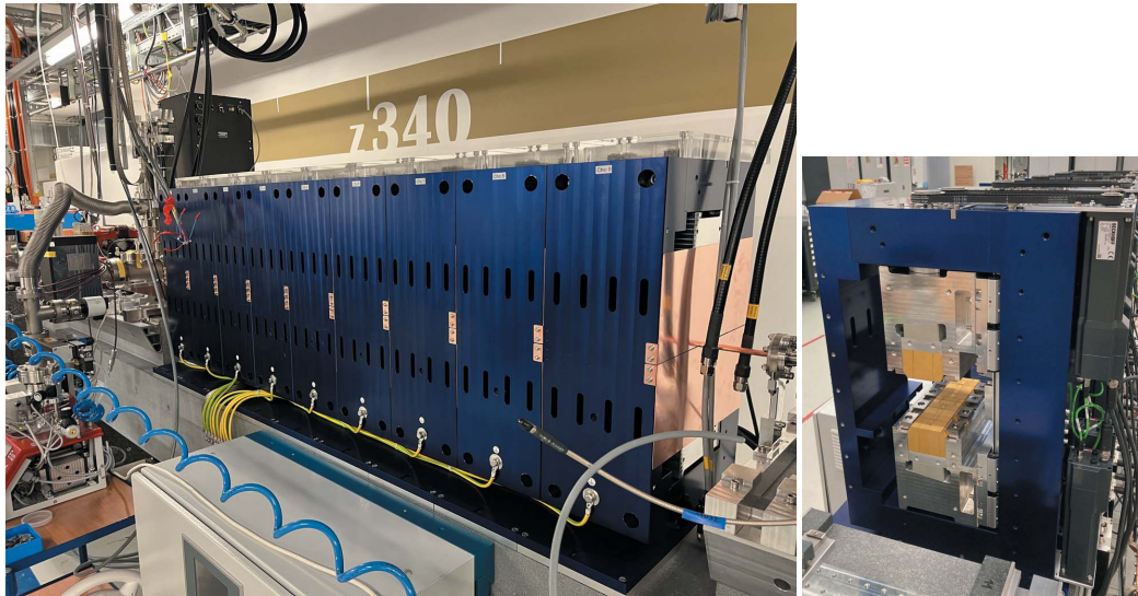
Figure 3.6: HERO modulator at Athos beamline, the left shows an installed modulator with eight periods. The right figure shows one period [64].
