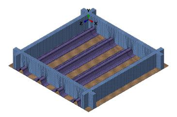
Fig. 11. FEA model geometry. For improved visibility, every second element is displayed.
