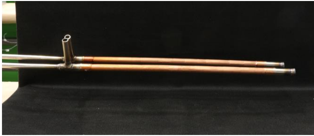
Fig. 3. The two conductors with steel jacket, copper termination and He inlet/outlet, before heat treatment.
