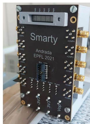
Fig. 14. Sensor board which comprises five 4 mm × 4 mm A-SiPM (Hamamatsu S14160/S14161 series). An amplifier (ADA4807) and a comparator (LT1394) are connected to each A-SiPM; the output of the comparator is made available through SMA connectors. The board can be interfaced with the board of Fig. 13 through coaxial cables.
