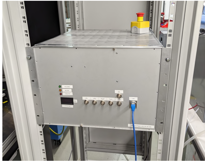
Figure 2.9: Picture of the nanosecond-pulsed high-voltage power supply with visible emergency shut-down button on top.
