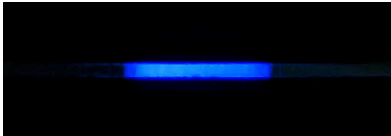
Figure 5.9: Image of the diffused VDBD plasma discharge with a membrane placed in the gap.
