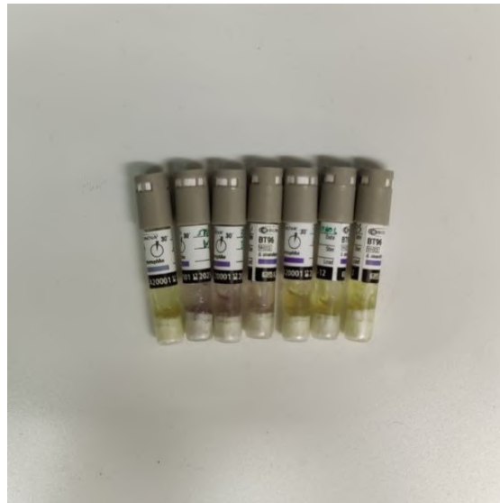
Figure 5.25: BT96 BI used for the sterilization experiments after 48 hours. The yellow vials correspond to unsuccessful treatments, while the purple ones are obtained after successful treatments.
