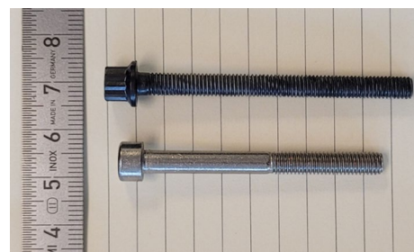
Fig. 2 Baseline stainless steel versus our novel CF/PEEK bolts for through-thickness insert fixture to a sandwich panel
