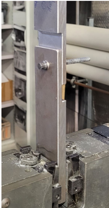
Fig. 5 Single shear test setup with a CF/PEEK fastener
