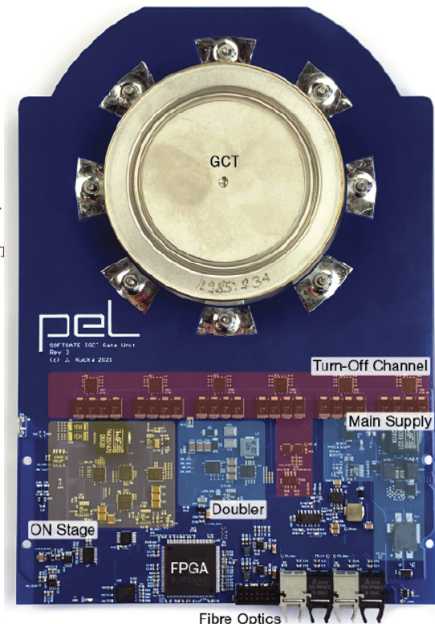
▲ Realized SOFTGATE gate unit
