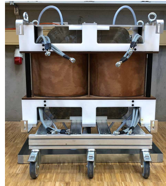
▲ 1 MW prototype of the 2-vessel MFT structure.
