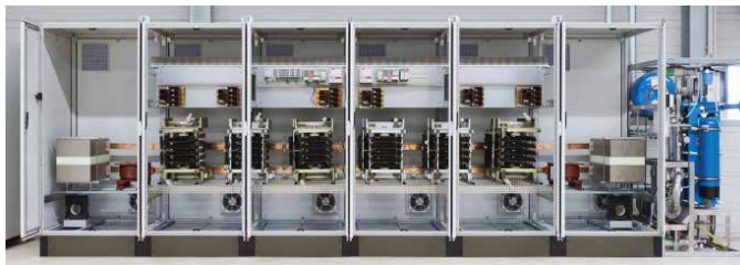
▲ 5MW, 1kHz 3PH DAB IGCT prototype at RWTH, Aachen
