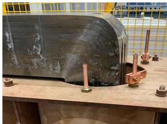
▲ MFT cores during assembly.
