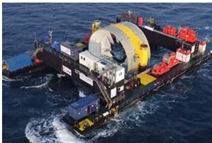
▲ EDF's OpenHydro deployment of the 2nd Turbine
