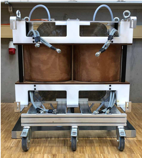
▲ 1 MW prototype of the 2-vessel MFT structure
