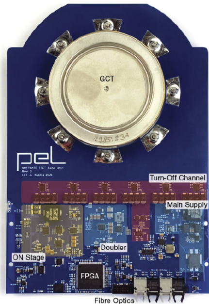
▲ Realized SOFTGATE gate unit [37]
