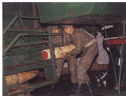
fig 103 | Firing exercise. Placing grenade and load in the ammunition elevator. Battery of Raposa, 1998
