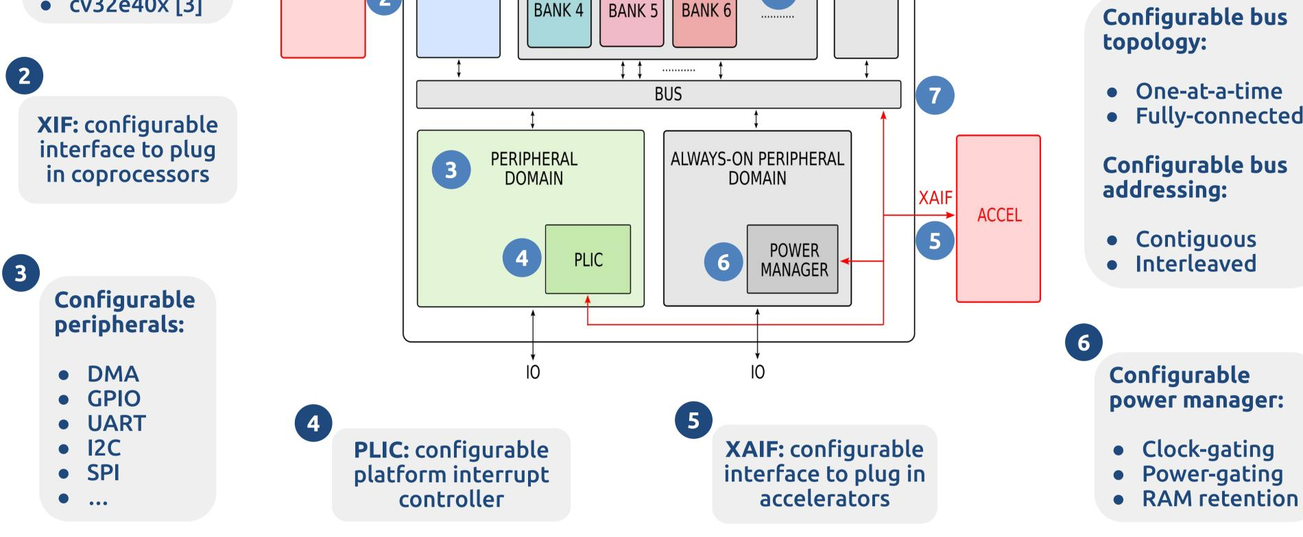
[1] Low-power, 32-bit, in-order RISC-V core with a 2-stage pipeline that implements RV32[E|I][M]C instruction set architecture. [2] High-performance, 32bit, in-order RISC-V core with a 4-stage pipeline that implements RV32IMFC[Xpulp] instruction set architecture. [3] High-performance, 32-bit, in-order RISC-V core with a 4-stage pipeline that implements the
