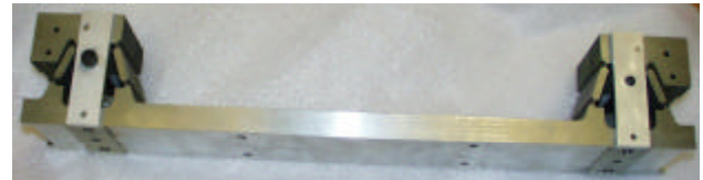
Figure 15: Detail of the flexural hinges on the mirror support
