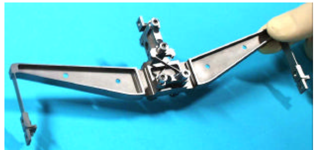
Figure 5: Electro-discharge machined coupling lever of the CCM
