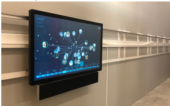
(b) View of the Linear Navigator, showing a portion of the rail the screen moves on
