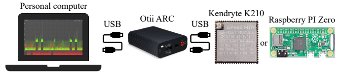
Fig. 11: Hardware setup for the energy consumption measurement. Otii Arc is connected to the computer using a USB cable. The main output of the Otii Arc is connected to the voltage supply input of the IoT wearable device. The computer’s USB port’s current is used to power the Otii Arc and edge AI platforms. The Otii desktop application enables us to measure and analyze the energy consumption of the edge AI platform. In our evaluation, we considered a development system that uses AI technologies embedded on a Kendryte K210 chip in different IoT wearable systems [77] or Raspberry Pi Zero.
