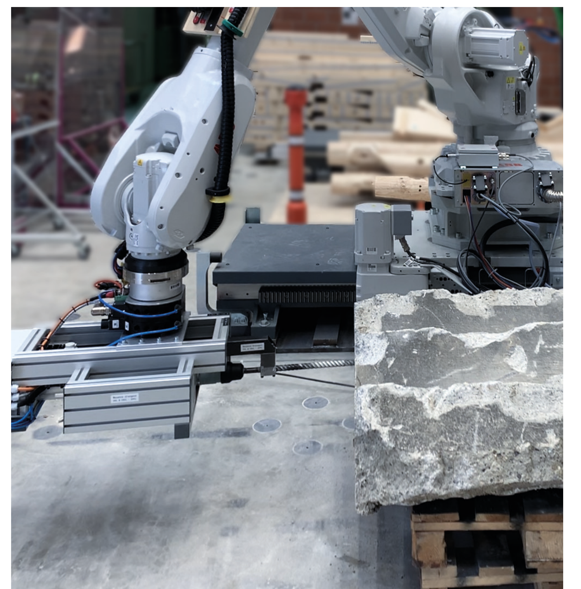
Concrete drill mounted on a 7 axis industrial arm, able to drill through concrete (rubbles) at full-scale
