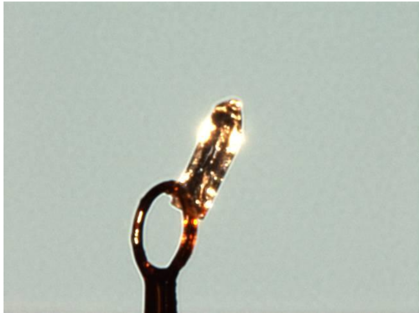
Figure S11: Image of the Crystal on the Diffractometer.
