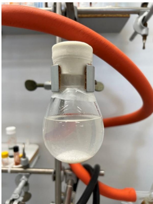
Photo S3. Reaction mixture before irradiation; partly insoluble N-benzylmaleimide could be observed on the bottom of the bulb
