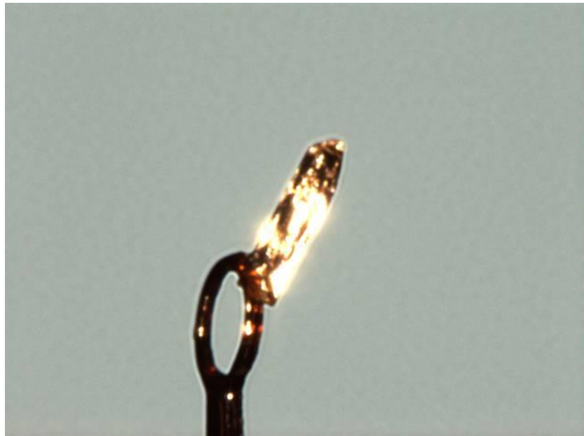
Figure S12: Image of the Crystal on the Diffractometer.
