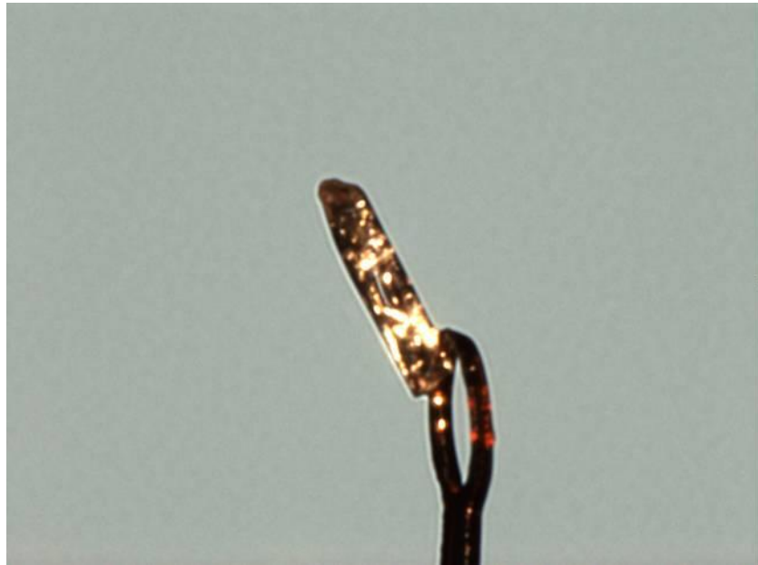
Figure S9: Image of the Crystal on the Diffractometer.
