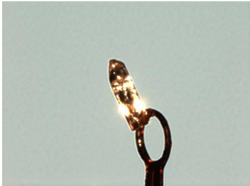
Figure S8: Image of the Crystal on the Diffractometer.
