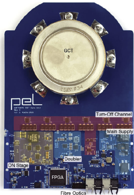
▲ Realized SOFTGATE gate unit [1]
