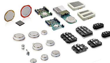
▲ Typical high power packages (Hitachi Energy)
