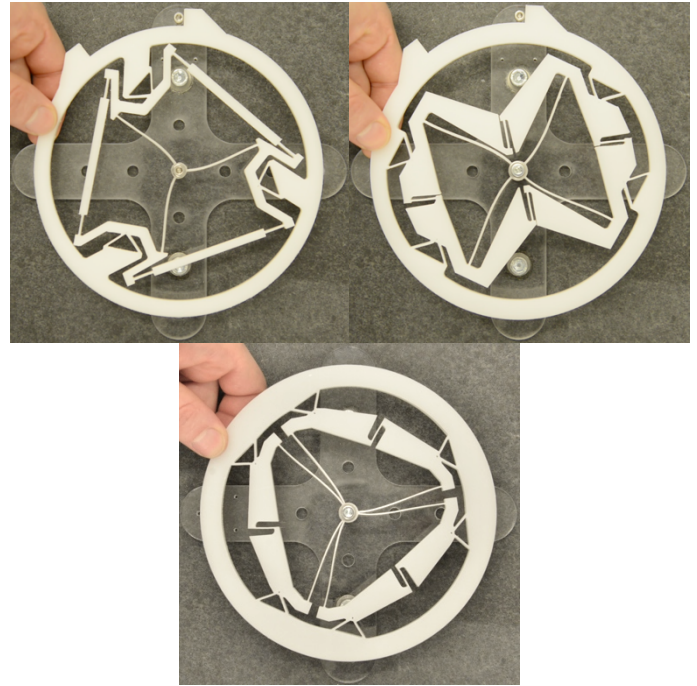
FIGURE 7: Mockups (POM, outer diameter of 150 mm) of (a) the TRIOVOT, (b) the QUADRIVOT and (c) the HEXAVOT. The inner body is attached to a fixed frame and the outer body is manually rotated.
