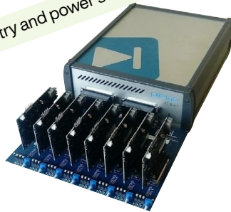
▲ RT Boxes used to host up to eight MMC control cards
