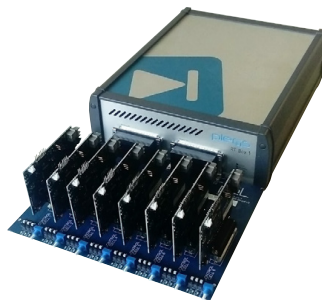
▲ RT Boxes used to host up to eight MMC control cards
