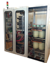
▲ 5 kV IGCT test setup and 10 kV DCT demonstrator under construction
