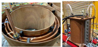
▲ MFT design optimization and 1 MW 5kHz MFT prototype
