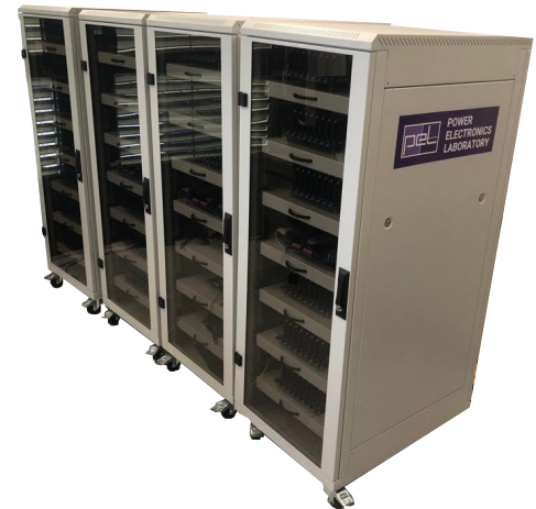
▶ Digital Twins - Four RT-HIL systems allowing for various topological reconfigurations
