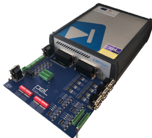
▲ RT Box hosting application
