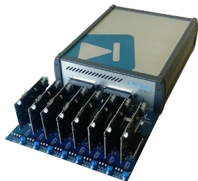
▲ RT Box hosting eight MMC sub-modules
