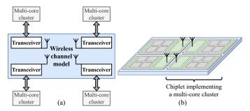
Fig. 4: Model of the wireless interconnect in system-level simulation, comprising one transceiver and nanoantenna per interfaced component (a), and emulated multi-chiplet system implementing a wireless chiplet interconnect (b).
