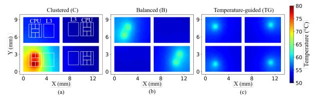
Fig. 5: Thermal maps of a 4-chiplet architecture executing MobileNetV2 on a wireless interconnect SoP at 2GHz, considering three task mapping configurations: (a) clustered, (b) balanced and (c) temperature-guided.
