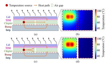
Fig. 2: Chiplet thermal simulation employing an existing thermal modeling technique (a, b) and the non-uniform method with 3D-ICE 3.1 [9] (c, d). For each simulation, heat flow through the layers, namely Interposer (Intp), Bump, Chiplet, Thermal interface material (TIM), and Lid from bottom to top, is shown in (a, c), and the thermal map for the layers in (b, d). Chiplets are delimited with dotted boxes.
