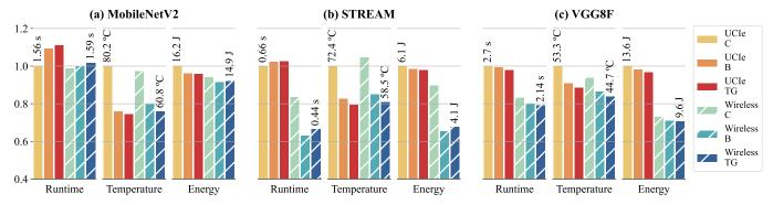
Fig. 6: Temperature, runtime and energy of the 4-chiplet system executing different workloads on 4 active cores at 2 GHz. Results are normalized with respect to the UCIe baseline employing the clustered (C) mapping strategy.
