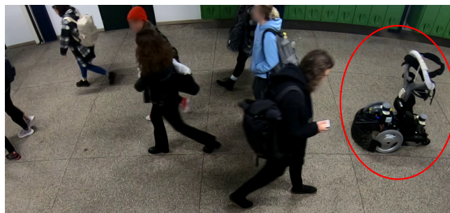
Fig. 8. In our experiments, the robot Qolo (encircled) drives in a busy corridor on EPFL campus by optimizing the learned objective J_{(a^1)} on-line.
