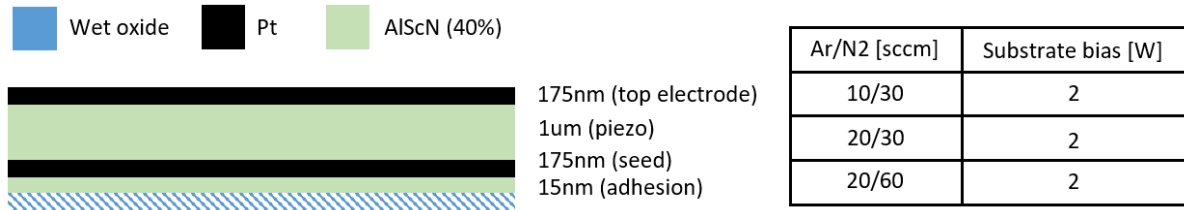
Figure 4: Materials deposited and parameters of deposition to characterize the effects of these parameters on the stress.
