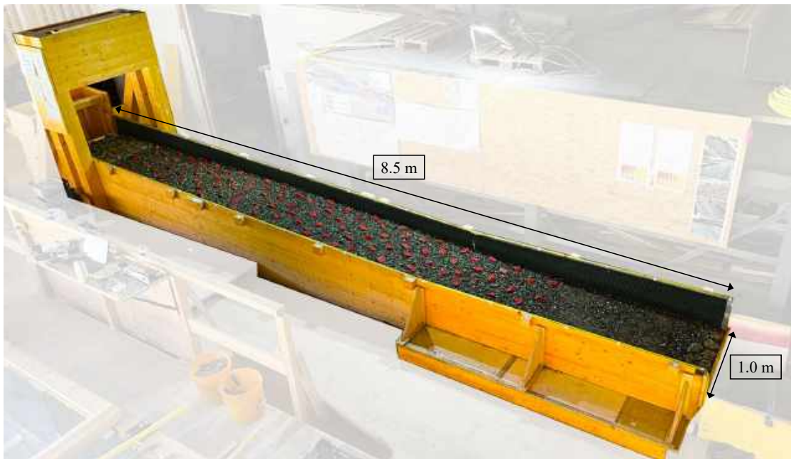
Figure 3.1: Photo of the model flume situated at Laboratorio 3D in the initial condition. Water will be run through flowing from left to right.
