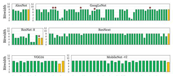
Fig. 9. Per-layer bitwidth of BOs (green bars for convolutional layers and yellow bars for fully connected ones) in the optimized benchmarks. IMOs are assumed to be reduced from the baseline 16-bit to 8-bit words, except for those in layers marked with a red star.
