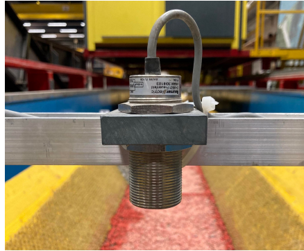
FIGURE 4.9 – Third ultrasonic sensor (USS) located in the riffle section.
