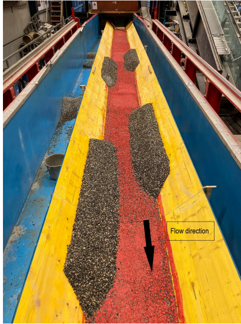
FIGURE 4.3 – Arrangement of the four sediment deposits prior to an experiment in the alternating configuration. The picture is taken in the upstream direction. The black arrow shows the flow direction.
