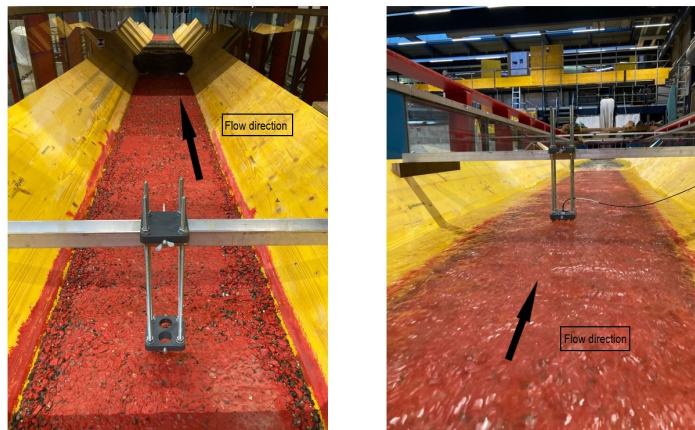
FIGURE 4.8 – Mount holding the UVP transducer at zero flow (left) and Q = 20 [L/s] (right). Both pictures are taken in the run2 section, looking in the downstream direction. The Black arrows show the flow direction.
