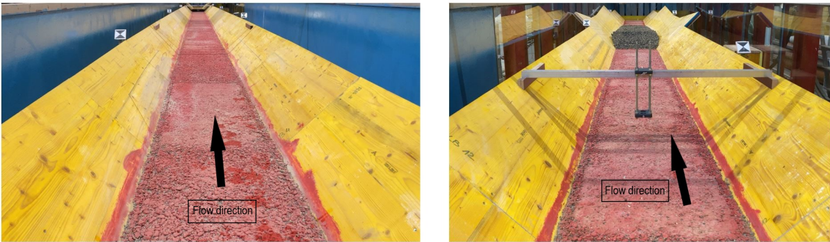
FIGURE 4.2 – Run section of the empty channel (left) and run2 and riffle2 sections of the empty channel, with the system for UVP measurements (right). Both pictures are taken in the downstream direction. The black arrow shows the flow direction.
