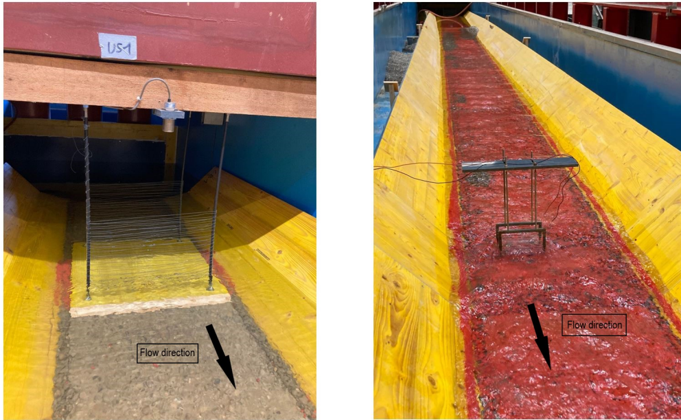
FIGURE 4.6 – Fixed (left) and mobile (right) apparatuses used to perform water hydrolysis. The fixed is located at the top of the channel, while the mobile is located in the run section. Both pictures are taken in the upstream direction. The black arrow shows the flow direction.
