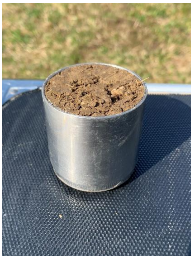
Figure 17: Example of cylinder collected in the top layer of grassland in Frick, 28 th of March.
