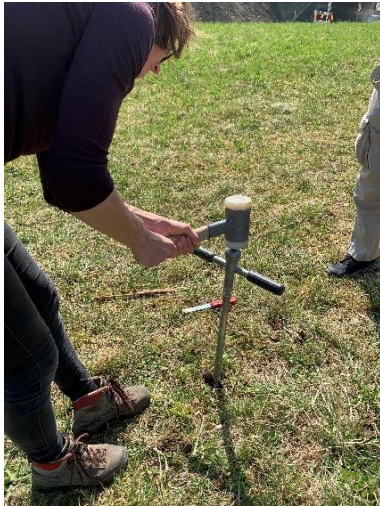
Figure 15: Use of the special auger for bulk density determination.
