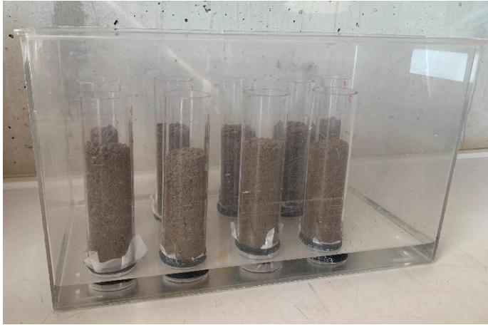
Figure 22: Soil samples progressively saturated with water for mWHC determination.
