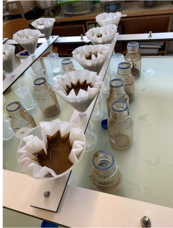
Figure 26: Extraction of the organic contents by filtration for microbial biomass determination.
