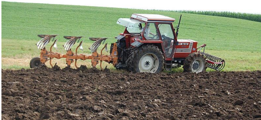
Figure 6: Moldboard plough commonly used for conventional tillage. Photo: Alfred Berner, FiBL
