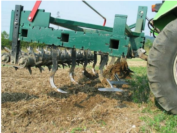
Figure 7: Chisel plough on the Ecodyn cultivator. Photo: Hansueli Dierauer, FiBL.
