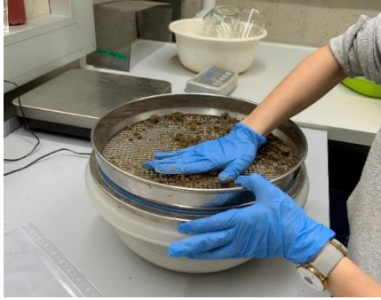
Figure 19: Soil sieving procedure. A sample of Aesch soil is shown.
