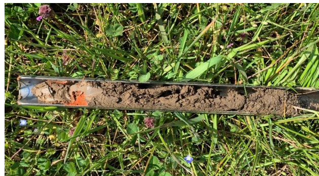
Figure 14: An example of a core extraction from the grassland plot G1 in Frick LTE, 24 th of March. One can see a clear difference in texture compared to Aesch soil. A piece of anthropogenic red brick is visible.
