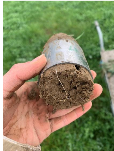
Figure 16: Example of a cylinder core extracted.
