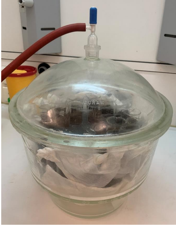
Figure 25: The desiccator used for chloroform fumigation. Here, the desiccator is shown after the 24 h incubation, connected to the vacuum for aeration.
