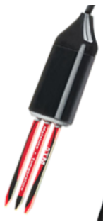
Figure 2.7: 5TM water content probe
