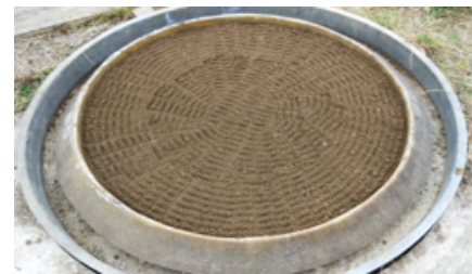
(b) Soil fill and surface preparation
