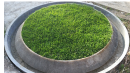
(c) Vegetated lysimeters at the beginning of measurements
