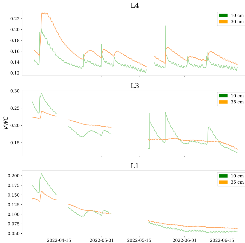
Figure 4.1: Comparison of VWC vertical dynamic between L1, L3 and L4. The green curve exceeding the orange one signifies that an upward gradient of water content forms in the soil column.
