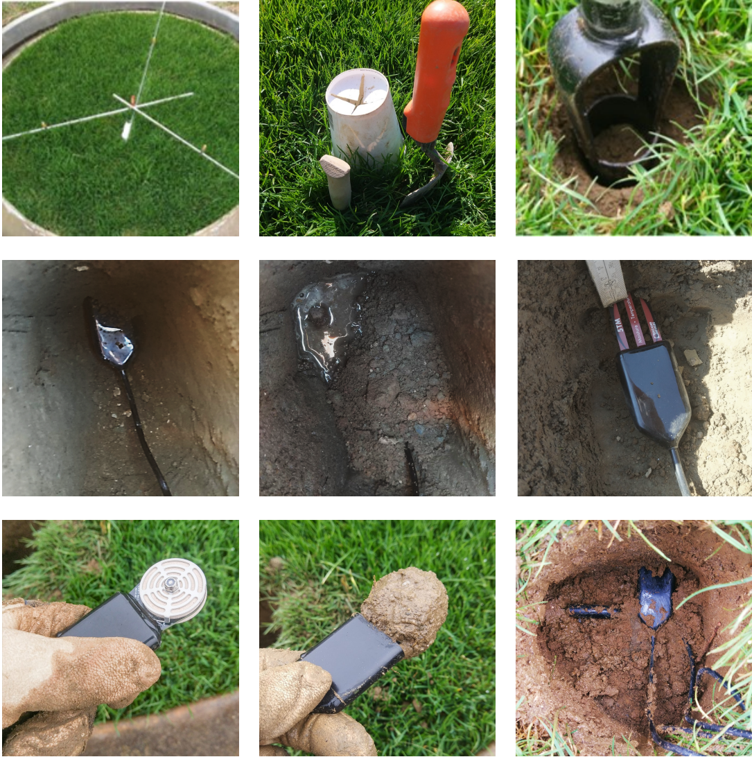
Figure A.3: Detailed procedure for 5TM water content sensor and TEROS 21 tensiometer installation
