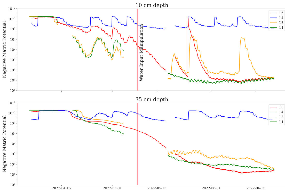
Figure 4.3: Matric potential comparison between lysimeters. The logarithmic negative values are displayed on an inverted axis. An upward curve corresponds to an increase of water availability
