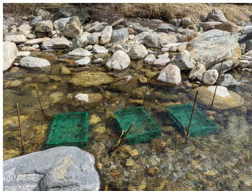
(a) Boxes containing glass slides for biofilm growth in river Ticino: The boxes had to be submerged and the flow rate had to be around 0.3 - 0.5 m/s.
