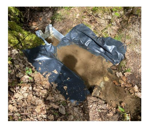
Figure 5: Alternative water-level sensor installation inside a V-notch weir box. In black, the tarp is connected to the inlet of the weir box and collect the flow coming from upstream.
