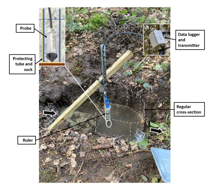
Figure 3: Detailed installation of a water-level sensor. Picture from location B7.
