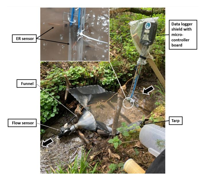
Figure 2: Detailed installation of a multi-sensor device. Picture from location B8.
