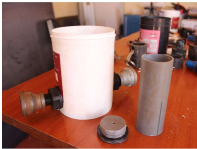
Figure 35: AkvoTur assemblage. From left to right: PVC vessel, PVC bottom plate, and PVC cylinder.
