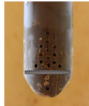
Figure 34: Chlorine containing cylinder, Kyuso. The dashed plate represents the disk where the tablets were placed.
