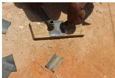
Figure 24: Heated pipe remodelling using a hammer.
