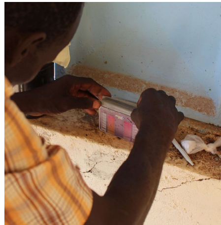
Figure 20: Kiosk operator taking a FRC measurement using the pooltester, Mitamisyi.
