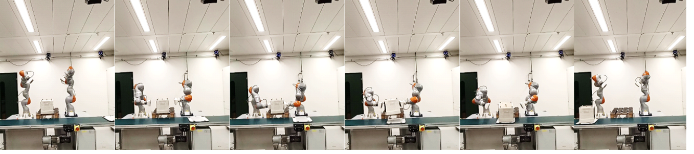
Figure 15: Snapshots of dual-arm grabbing and object tossing (white cubic box) onto a moving target (white tray on conveyor belt). At first, the robots wait for the target to reach the estimated state-to-go before moving toward the object to grab it and toss it to the target moving on the conveyor belt. From left to right, the snapshots show the dual-arm system waiting, approaching the object, grabbing the object, tossing the object, intercepting the moving target and landing, and both moving together.
