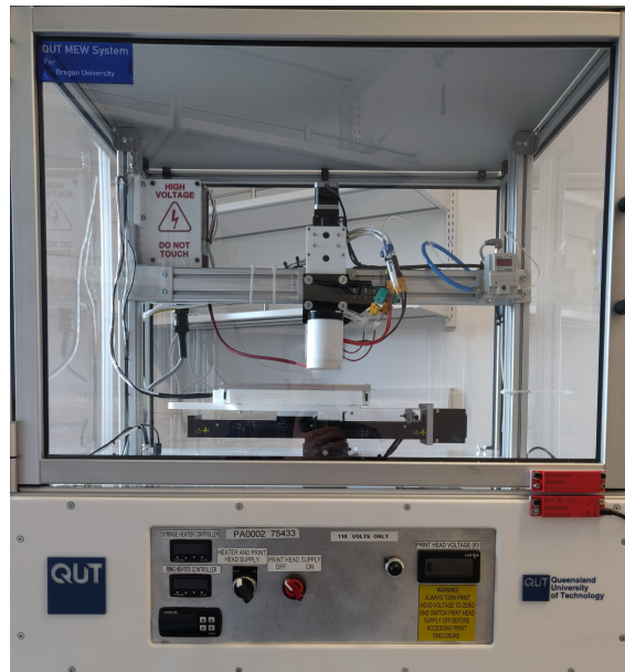
Figure 2.8 Example of a MEW system: The Queensland University of Technology MEW system
