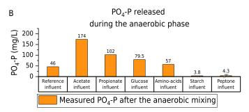
Figure 6.2: Effect of different carbon sources on bioreactor RB
