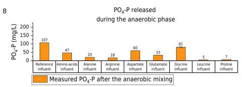
Figure 6.4: Effect of individual amino acids on bioreactor RA
