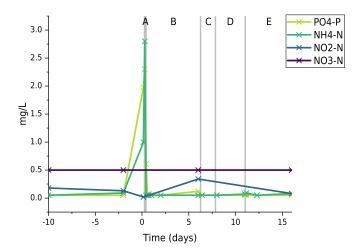
Figure 2.2: **Effect of an operational failure on the nutrient removal**  $PO_4^{3-}$ ,  $NH_4^+$ ,  $NO_2^-$ , and  $NO_3^-$  were measured in the effluent before and after an operation failure of the bioreactor.
