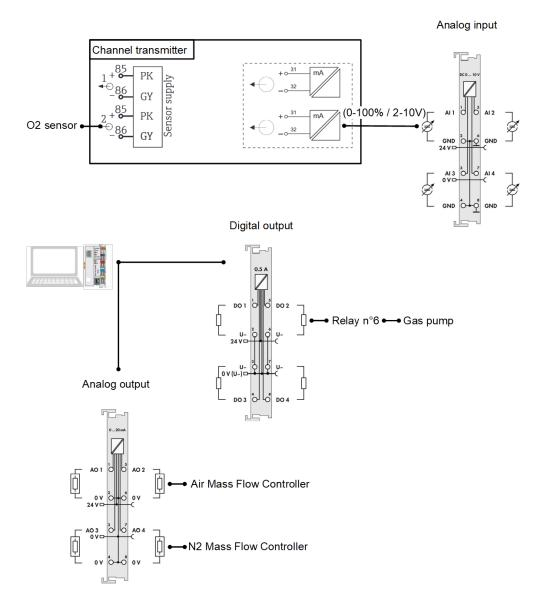
Channel transmitter: Liquiline CM442-19W0/0, Endress+Hauser® with a  $500\Omega$  resis-
