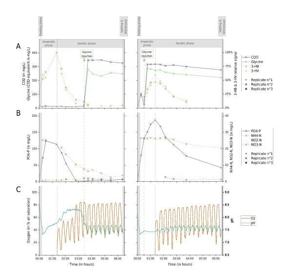
Figure 6.7: Effect of a glycine addition in the anaerobic and aerobic phases during different SBR cycles of bioreactor RA
