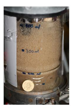
Figure 2.1: Picture of the bioreactor setup used for the Stable Isotope Probing
