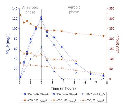
Figure 6.6: **COD** and **PO<sub>4</sub>-P** concentration during **SBR** cycles in bioreactor **RA** treating influents with different glycine concentrations.
