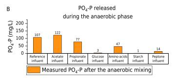
Figure 6.3: Effect of different carbon sources on bioreactor RA
