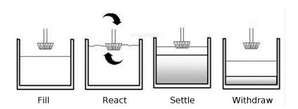
Figure 1.1: Four different phases of an SBR operation
