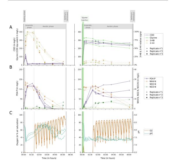
Figure 6.8: Comparison between SBR cycles performed on bioreactor RA with the reference influent and with an influent containing glycine as sole organic carbon source
