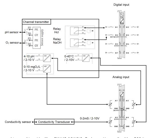
Channel transmitter: Liquiline CM442-19W0/0, Endress+Hauser® with a  $500\varOmega$  resis-
