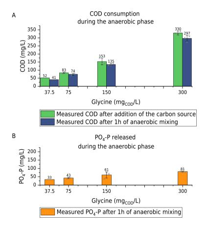
Figure 6.5: **Dose-dependent effect of glycine on bioreactor RA**RA's reference influent contains a mixture of acetate and propionate as organic carbon sources. The different modified influents containing glycine as a sole organic
