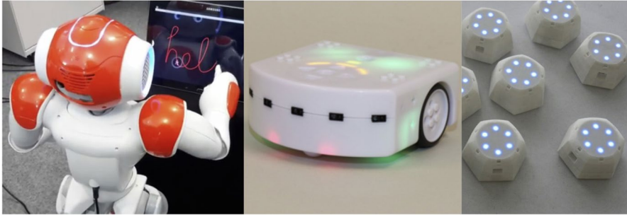
Fig. 1 Different categories of robots used for education: From left to right: NAO (Lopez-Caudana et al., 2022), Thymio (Chevalier et al., 2016) and Cellulo (Özgür et al., 2017b) robots used for education. Thymio and Cellulo are both educational robots, with Thymio being a tabletop platform for Computer Science (CS) and Computational Thinking (CT) skills acquisition, while Cellulo is a robot aiming to enhance and mediate the acquisition of disciplinary content via students' interaction. NAO belongs to other category of social robots, more expensive and less used in classroom settings, used for specific learning contexts (Lopez-Caudana et al., 2022)
