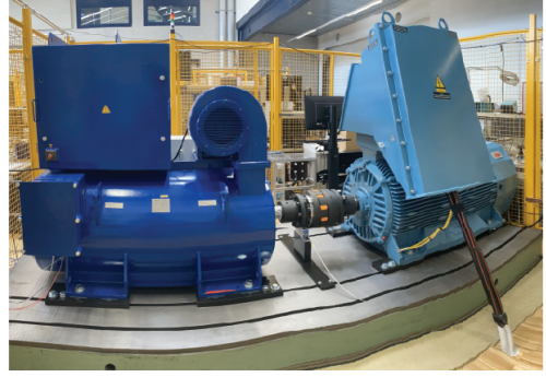
Fig. 11. Picture of the Medium Voltage (MV) test bench, in dark blue the SM and in light blue the Induction Machine (IM). Both machines are rated at 500 kW and are connected on the same shaft.
