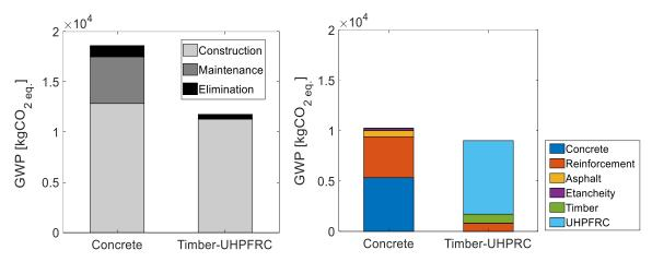
Figure 4 Environmental impact of bridge designs. A) Total impacts over the bridge service duration. B) impacts of the construction of the bridge superstructure.
