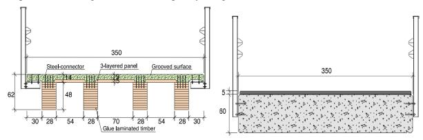
Figure 3 Alternatives: A) timber-UHPRC; B) Reinforced-concrete bridge.
