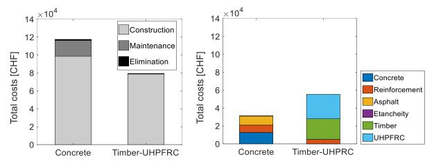
Figure 5 Life-cycle costs of bridge designs. A) Total costs over the bridge service duration; B) Construction costs of the bridge superstructure.
